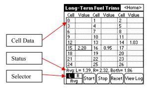
This screen is used to collect the LTRIM's (Long-Term Fuel Trims). These are the amounts by which the computer has increased or decreased the amount of fuel delivered under different conditions, in order to maintain a perfect 14.7:1 air/fuel ratio, as seen by the O2 sensors. Each set of conditions is called a "cell". Cell 16, for instance, is normally used when the car is idling.
